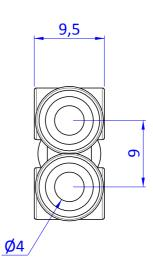
THE PROPERTY OF THE DRAWING IS ESTABILISHED BY LAW. IT IS FORBIDDEN TO PRODUCE OR SHOW IT TO THIRD PART. WITHOUT A WRITTEN AGREEMENT DESIGNED FROM REVIEW **FPS Automation** Α DATE WEIGHT 0.006Kg 24/08/2016 GENERAL TOLERANCE DESCRIPTION Format Α4 CODE UNI - ISO 2768 CA.12.05.004 UNI 936-76 CA.12.05.004 CLASSE f
